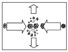
In the intense turbulence surrounding the blade, particles hit one another at high speeds and are further broken. The area where these collisions occur, beginning at the blade and extending out about two inches, is called the "zone of attrition".
