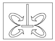
Beyond the zone of attrition, the now broken material is throughly mixed and particles are dissolved or dispersed by the laminar flow set up by the blade. The flow is separated at the vessel's wall ensuring complete circulation.
