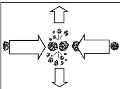
In the intense turbulence surrounding the blade, particles hit one another at high speeds and are further broken. The area where these collisions occur, beginning at the blade and extending out about two inches, is called the “zone of attrition”.
