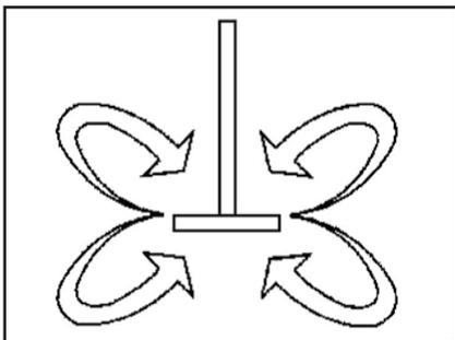
Beyond the zone of attrition, the now broken material is thoroughly mixed and particles are dissolved or dispersed by the laminar flow set up by the blade. The flow is separated at the vessel's wall ensuring complete circulation.
