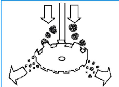
Particles hit the blade and are broken apart.
