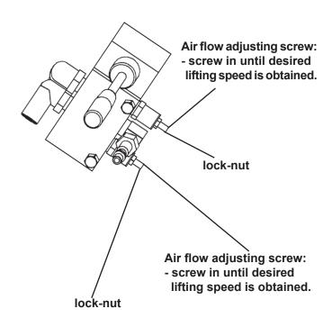
Once desired raise & lowering speeds are obtained, tighten lock -nuts.
