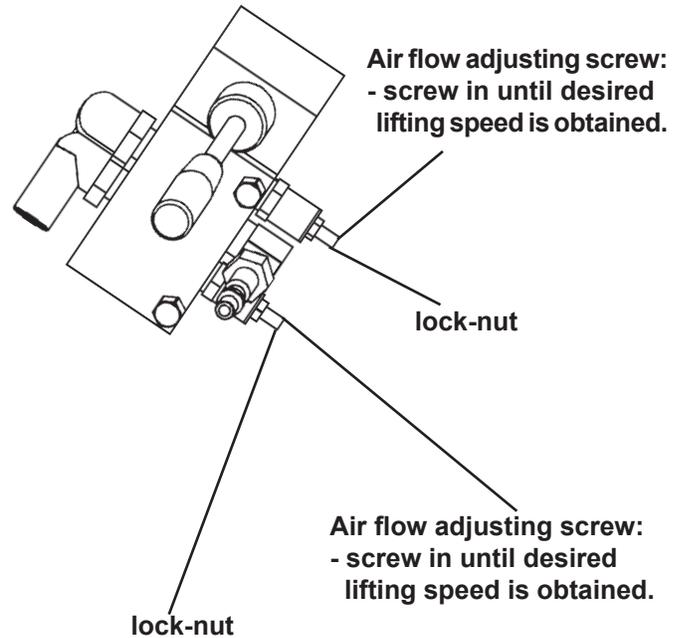
Once desired raise & lowering speeds are obtained, tighten lock -nuts.
