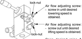
Once desired raise & lowering speeds are obtained, tighten lock-nuts.
