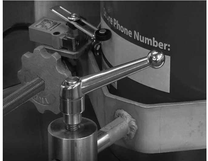
Figure 5. Container Limit Switch in the closed position
